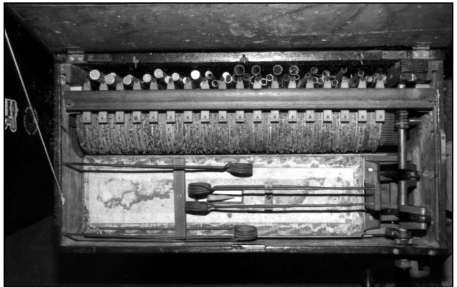
Figure 13. The interior of an 18-key Hinton hand organ clearly shows the crankshaft on the right side, with the barrel between the pump and the pipes, which speak in the front.
